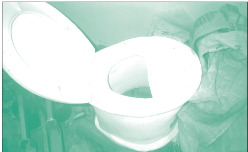
Locally produced toilet bowl for urine separation in Kisumu, Kenya
