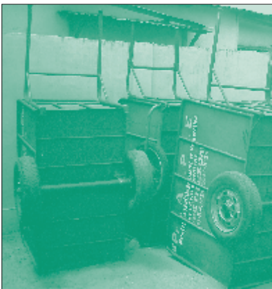
Simple technology: Manual push-carts for refuse collection in Benin
