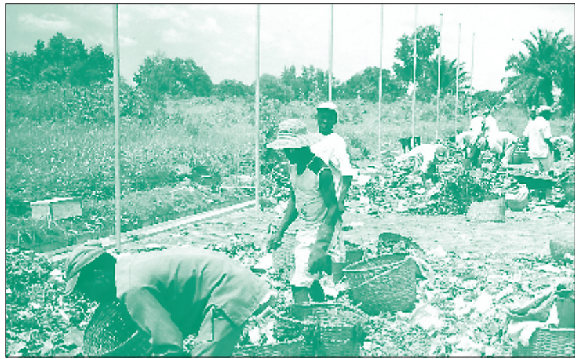
Manual sorting to identify waste composition and fractions in Cotonou, Benin
